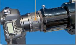
DSLR camera. CCD cameras might need custom adapter tubes, as I was advised by Pacific Telescope Corp. that the flattener-to-sensor distance must be within a millimetre of 75 millimetres for a truly flat field image.
