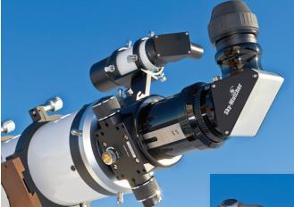
**VISUAL vs. PHOTO** For visual use, a step-down ring attaches to the 3-inch-diameter focuser, providing a standard 2-inch visual back. For photo use, seen here, another adapter ring allows the field flattener to attach to the focuser. This flattener has a camera adapter tube with T-threads for accepting DSLR T-rings or CCD camera heads. All adapters are included with the Esprit 120.
